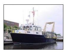
The John F Looney is a 46 ft stern loading buoy tender. She is ideal for coastal research projects, mooring work, and recovery. This vessel is a steel construction; with a beam of 16'2" draft of 5'1" and a cruising range of 440 nautical miles.
